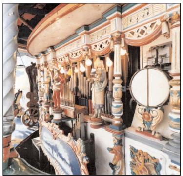
Figure 4. The Gavioli mounted in a smaller gallopers post-conversion to the 89 VB scale, probably in the 1960s. The violin pipes are removed from the organ in this photo. Photo courtesy of Rosie Screeton Armitage.
